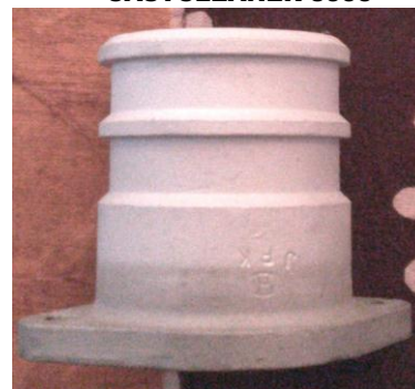
SS Casting before Cleaning
